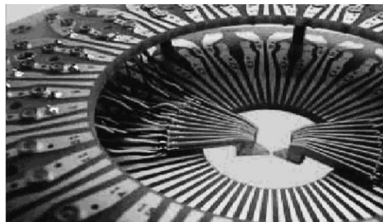
Figure 4. Keithley S600 Series low leakage probe card.
